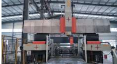
01 FLATNESS Processed on a large CNC milling machine for flatness.
